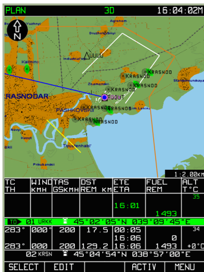
3-66: MENU/PLAN sub-mode view prior to activation
