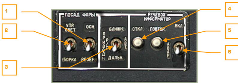
2-41: Landing lights and voice warning ("Betty") control panel.
