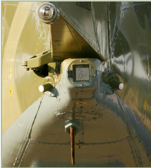
1-6: The tail of the Ka-50. The white navigation light is located at the top of the image. The L-140 laser sensor system is in the center and various IFF antennas are located to each side and below
