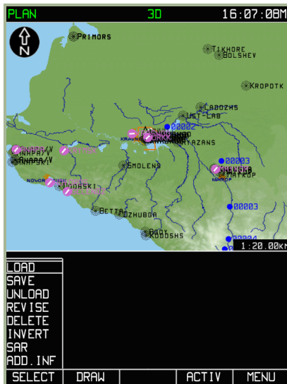
3-67: Selecting MENU/PLAN/LOAD sub-mode
