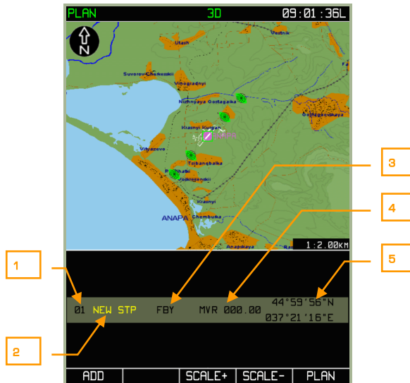
3-29: MENU/PLAN display when waypoint entry mode is entered
