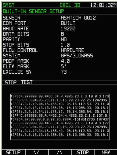
3-101: SYST page during testing of the GNSS sensor and its communication channel
