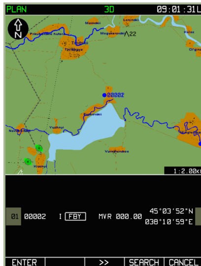
3-35: MENU/PLAN sub-mode display after successfully completing a navigational point search by use of callsign
