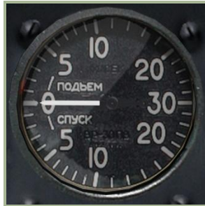
2-16: Vertical Velocity Indicator (VVI)
