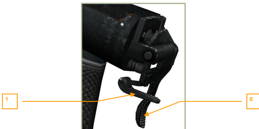
2-5: Weapon (large) and Cannon (small) triggers in default position – Release Weapon trigger operates
